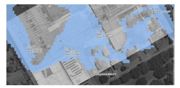
Considering this information, the minimum habitable floor levels have been designed to the Flood Planning Level (FPL) of 575.971 R.L which includes the 500mm freeboard above the highest anticipated flood level for the allotment.
